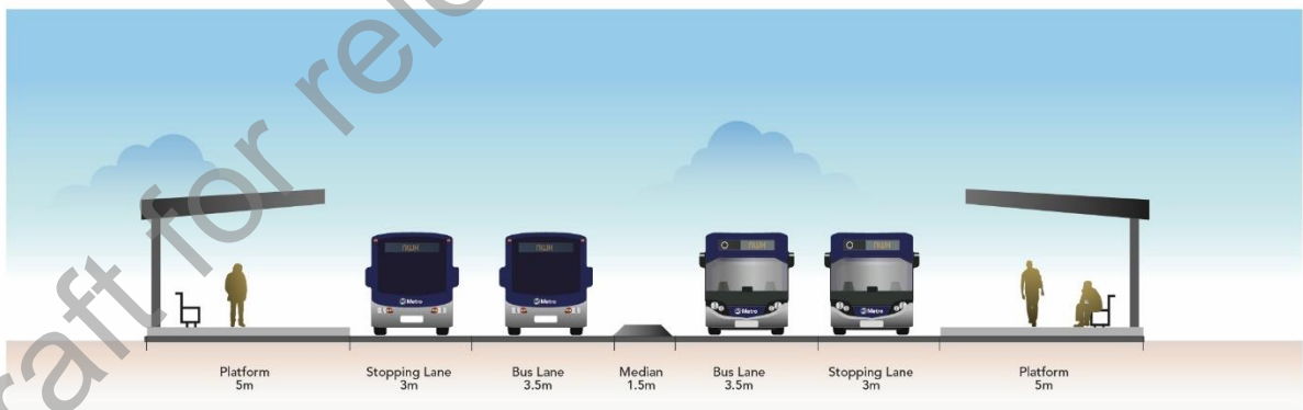
Figure 6.7 - Bus station cross section (Local RTN)
