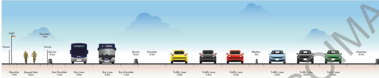
Figure 6.3 - Separated busway cross section
