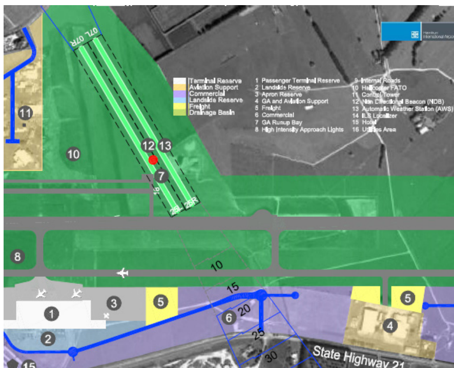
FIGURE 6-2 GRASS CROSS RUNWAYS – POSSIBLE RE-ALIGNMENT
