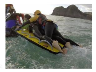
**Note:** Operator to ensure that RWC is facing into oncoming waves after each rescue is conducted, if not the risk of capsizing the RWC and injury to the patient is increased.
