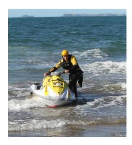
When beaching the RWC, always step off on the seaward side, so that a wave will not push or roll the RWC onto you.
