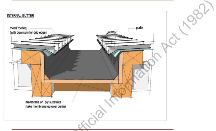
Where gutters penetrate external walls to discharge into rainwater heads, the full width of the gutter shall extend through the parapet into the rainwater head and terminate with an end drip-edge.
