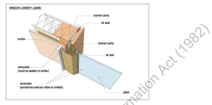
This illustrates the 3 stages of a successful weather-tight junction, both for the window to cladding junction and the glass to window frame junction.
