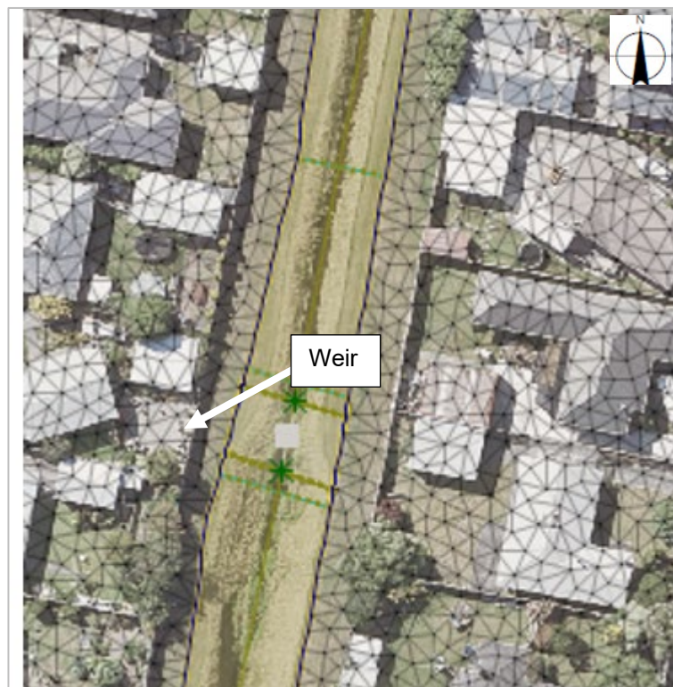
Figure 7-15 Model development with weir location identified
