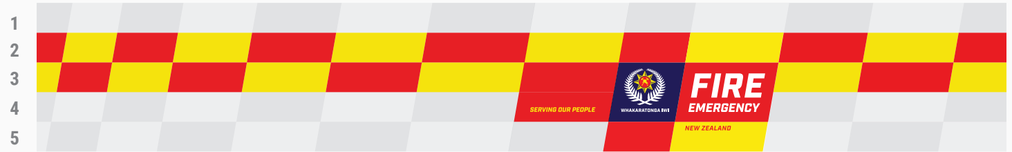
RIGHT SIDE – 'FIRE EMERGENCY' should always point to the front of the vehicle
