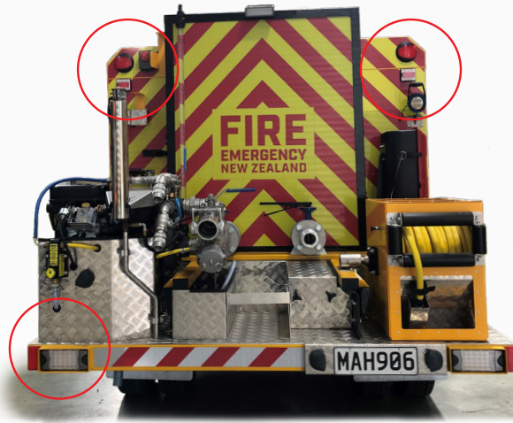
Daytime photo showing the non-reflective around the require lamp
