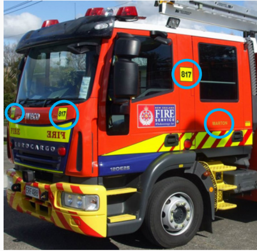
Remove non-approved call sign number on grill, remove call sign number on 'B' pillar, remove old station name circled in blue. Remove 'FIRE' & 'ERIF' off the grill.
