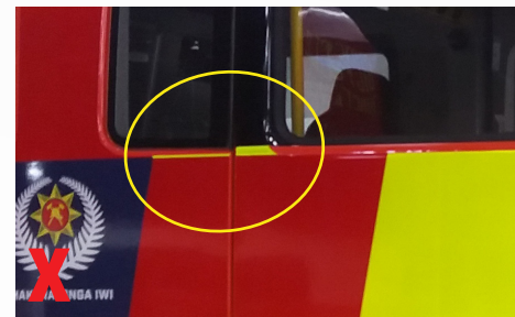
Do not apply small pieces of vinyl into areas that break the Battenberg pattern.
