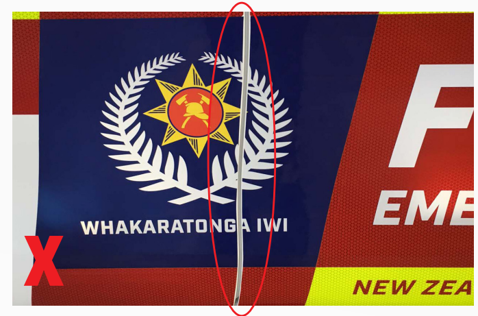
Do not allow the crest to be interrupted by door openings/panel gaps.
