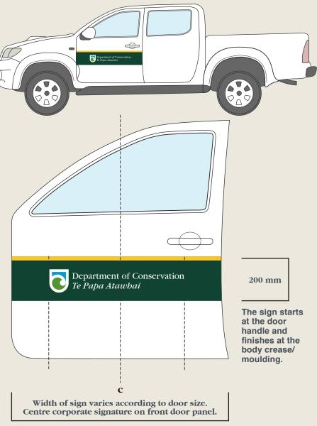
The decal is supplied at 1300 mm x 200 mm. Trim off excess if too long and smooth down edges. The decal should be applied to both front doors.
