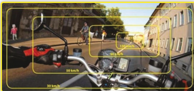
Illustration 1: Speed and field of vision (Ministry of Infrastructure, 2015)
