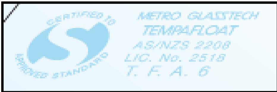
Figure above: sample of safety glass markings (Metro Glass Tech)
