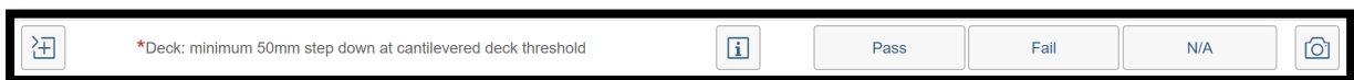
Figure 122. Checklist line item 'Deck: minimum 50mm step down at cantilevered deck threshold'
