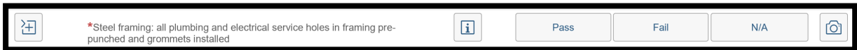
Figure 173. Checklist line item ‘Steel framing: all plumbing and electrical service holes in framing pre-punched and grommets installed’
