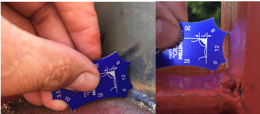
Figure 159. Example of a simple tool available from most engineering tool suppliers to check weld size. The photo on the right shows a weld which is too small.
