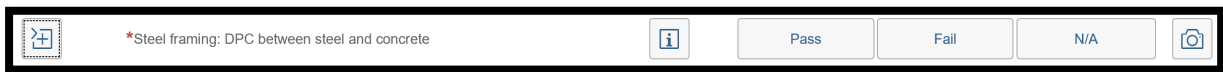
Figure 149. Checklist line item ‘Steel framing: DPC between steel and concrete’ All steel framing against concrete must have DPC separation.
