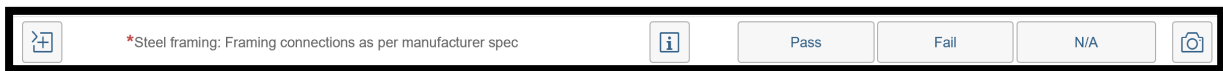
Figure 148. Checklist line item ‘Steel framing: Framing connections as per the manufacture specs’ All top plate, studs, nogs, lintels must have fixings in accordance with the manufacturer specifications.
