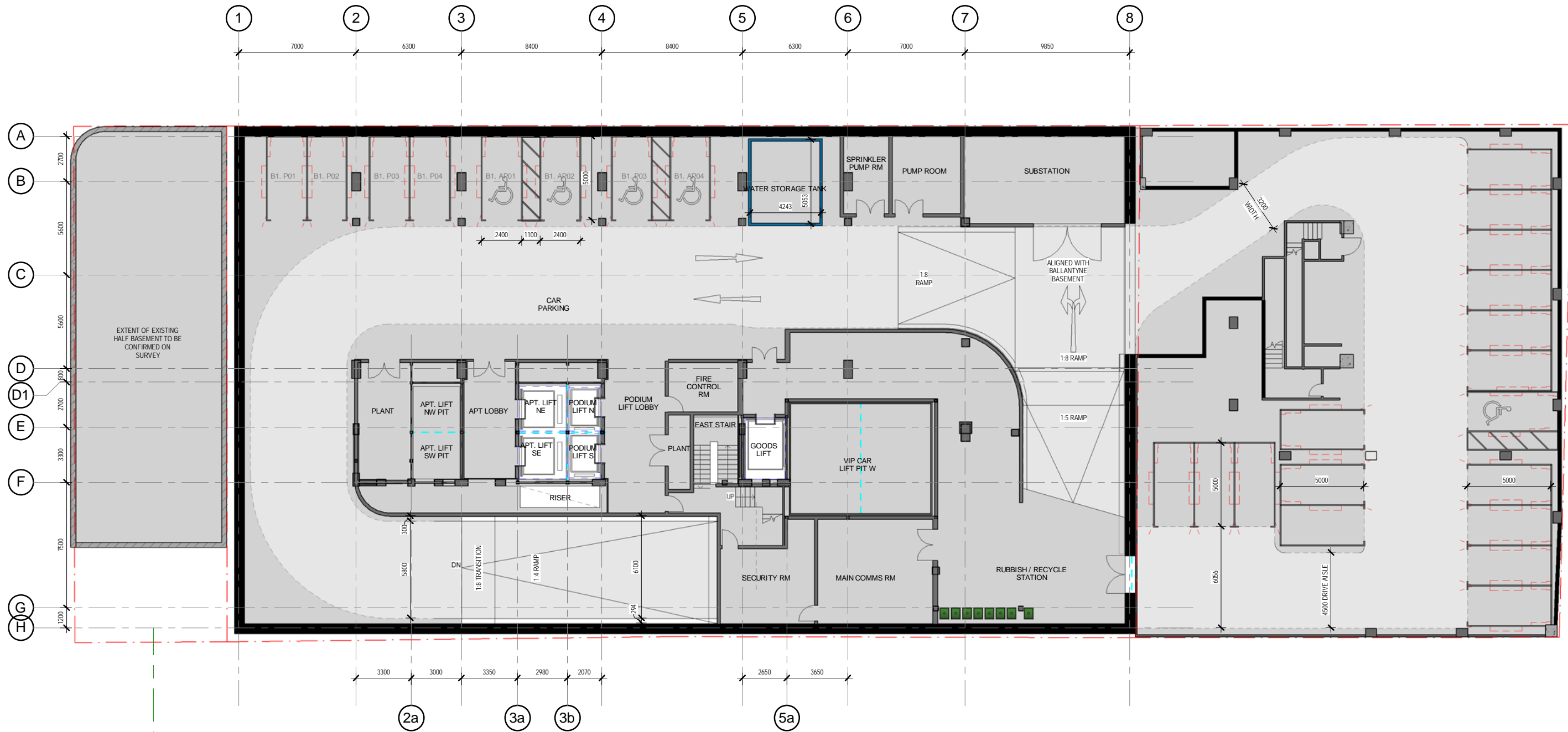
1 B1 - BASEMENT SERVICE FLOOR SCALE 1 : 125
