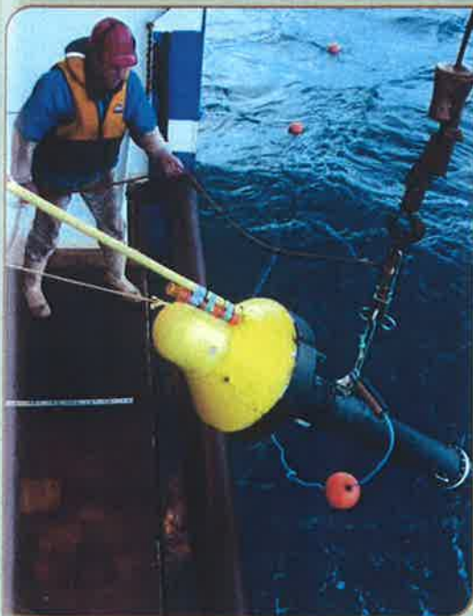
Tony Reiri deploys a Carioca surface drifter buoy off Tangaroa during SAGE.
