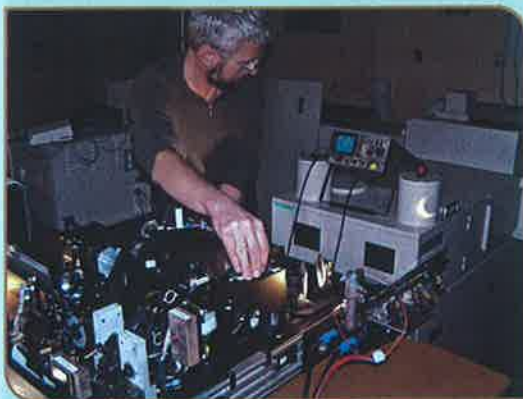
John Robinson using the Fourier Transform Spectrometer at Lauder to measure greenhouse gas columns (the total amount of a gas between the ground and the top of the atmosphere).
