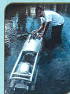
Postdoc Koustuv Debnath using the NIWA-designed and built in situ biophysical flume to measure streambed erosion.
