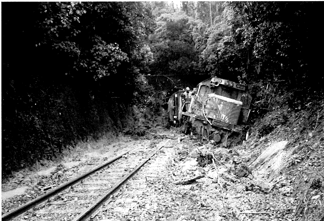
Figure 22 – Resilience and Slopes in Action – Wairarapa passenger train derailed after exiting a tunnel and hitting a rainfall-triggered landslide in 2009, stranding about 300 passengers in the tunnel for several hours and closing the line for several days.
