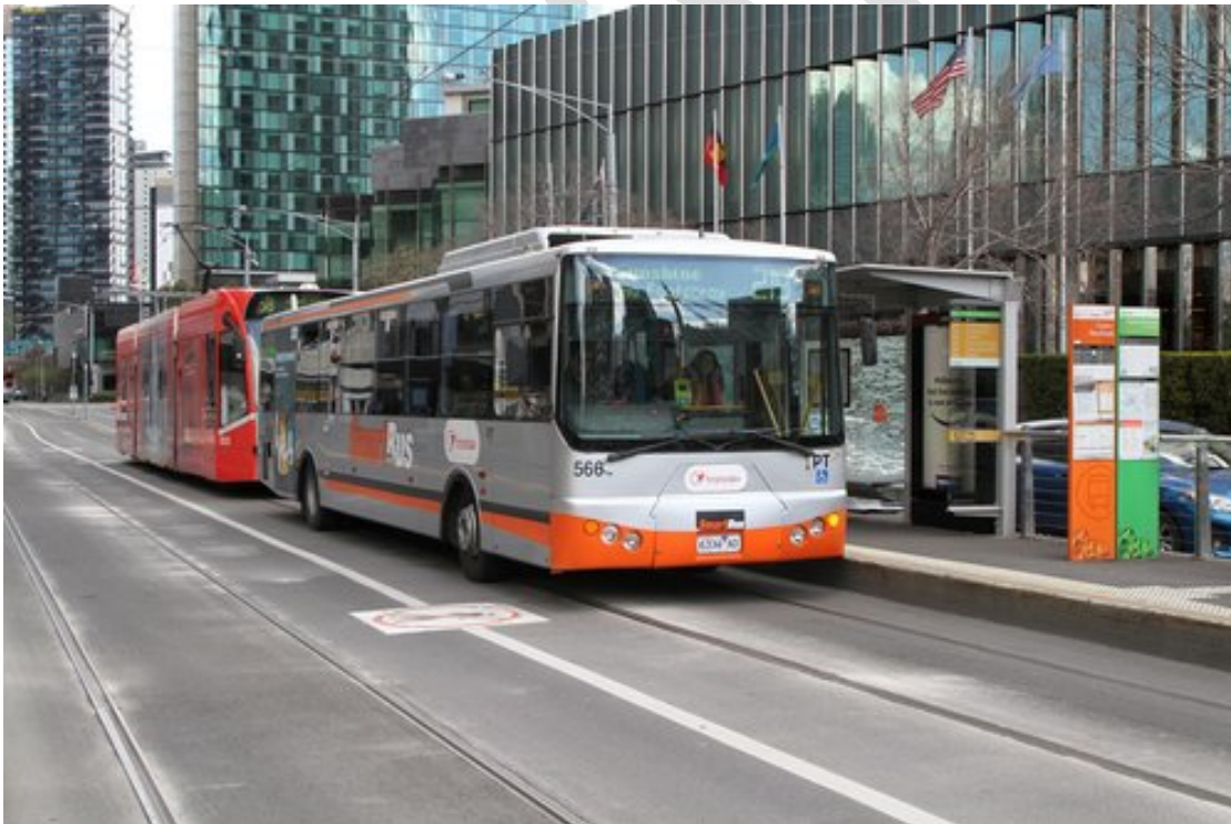
Example of bus and tram services sharing the same platform at Queens Bridge Street, Melbourne (image source: Marcus Wong )
