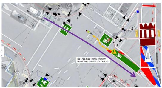
Figure 4-2: Through-cyclist deviating to avoid cyclist waiting in hook turn box
