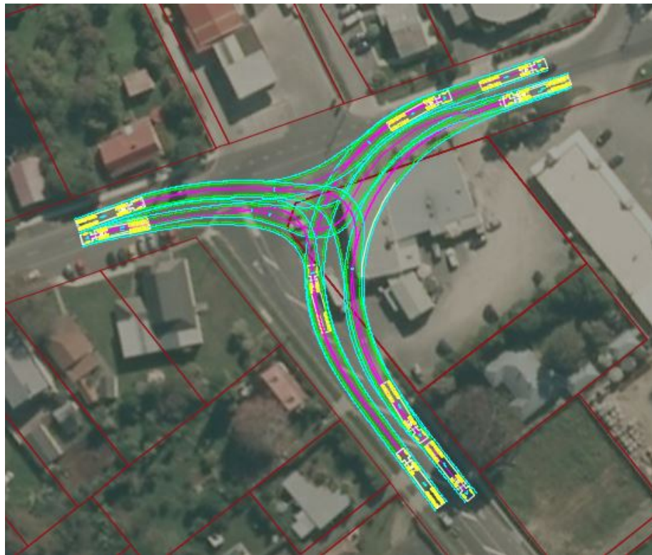
Figure 2-2: RTS tracking to check possibility of right turn bay with relocating 4 Square
